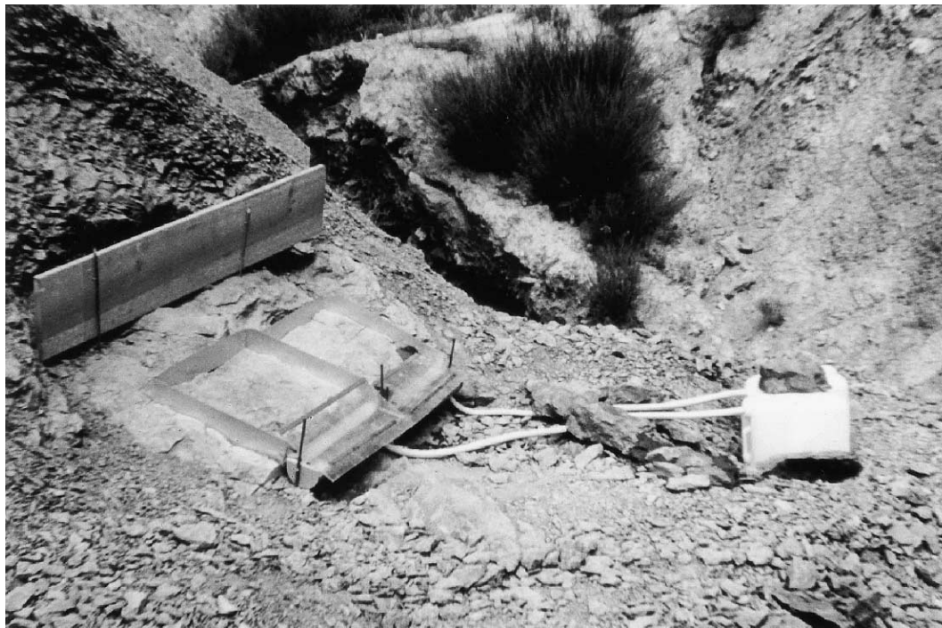
Fig. 3. Weathering plots (50×50 cm) equipped with Gerlach troughs to collect water and sediments, which are conveyed to a PVC jug.
